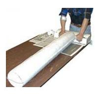
When this first wrap has cured enough to be hard, but not to a full cure, debag the tube and remove the breather and release. They should come off without much trouble and the breather may be usable again. Proceed to the second layup of the veil, following the same proceedure as for the base layup and bag it. Once the second layup has partially cured, debag the tube and remove the breather and release. Set aside to fully cure.
