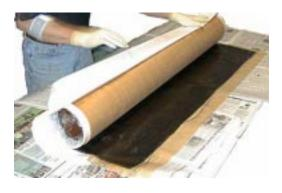
wraps around the tube. Once your wrap the cloth around, carefully inspect the entire surface to make sure you don't have any bubbles or wrinkles. The cloth should be stretched tightly and should overlap only slightly. Ideally, the overlap should be only the frayed edges of the cloth so that it makes the same thickness at the seam as the solid cloth on the rest of the tube.
