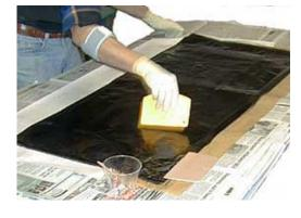
to make sure the cloth is tight. Peel back the freezer paper as you roll to make sure it doesn't get under the cloth as it
