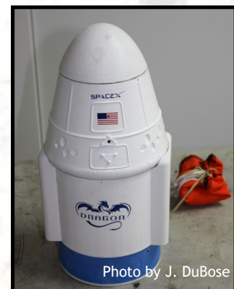
Dragon capsule and trunk. Printed early in the project with ABS filament
