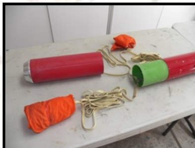
FBLP Booster showing main & drogue with "y" harness
