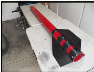
FBLP Booster with 3 fin Rousetech fin can
