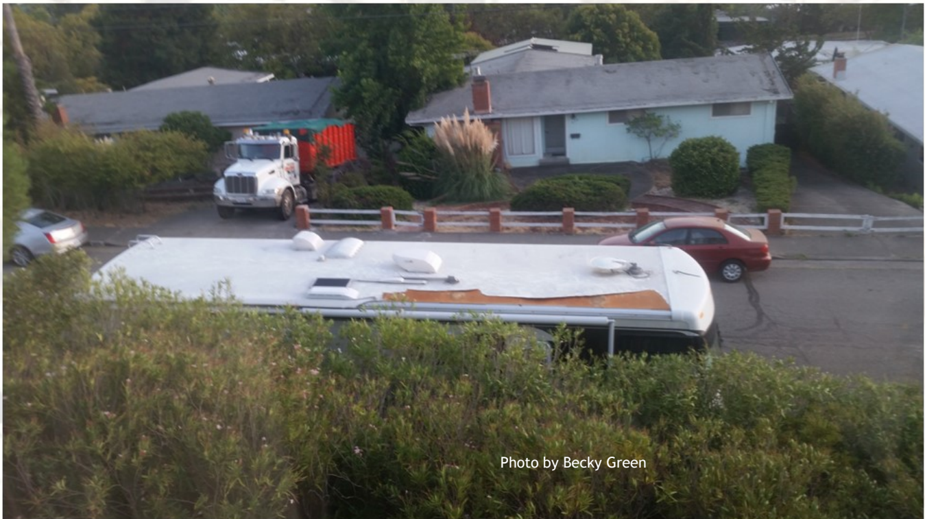
Big chunks of the Filon/fiberglass roof missing
