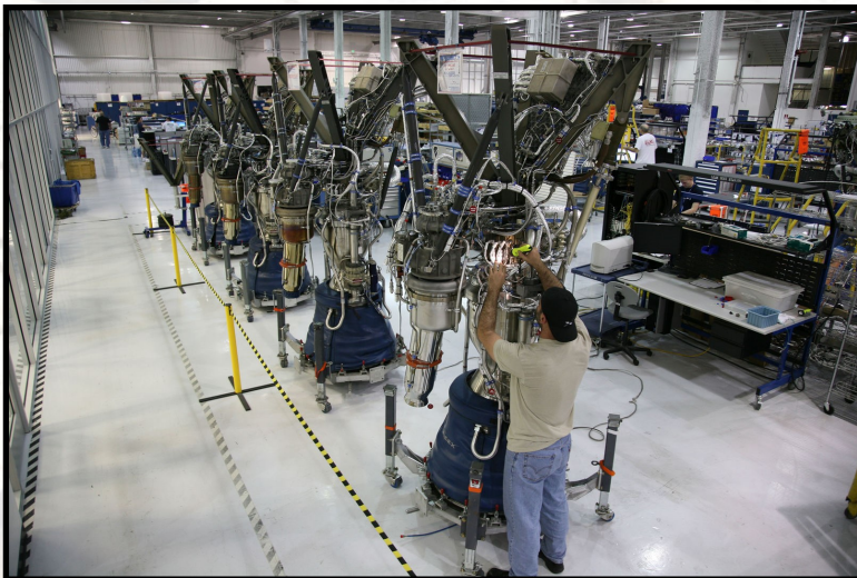
Assembling Merlin Engines
