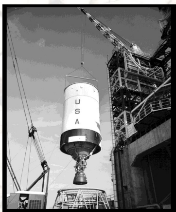
Left: An S-IVB is hoisted onto the test stand prior to fueling and firing.
