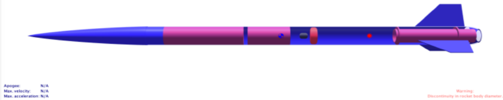
ARLISS-K - the lesser Mojo Length 174 cm, max. diameter 7.94 cm Mass with no motors 2440 g
