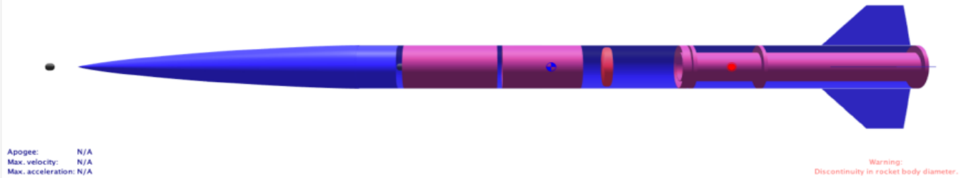
the greater Mojo Length 282 cm, max. diameter 15.6 cm Mass with no motors 9401 g
