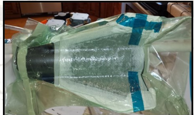
Figure 3: Fin attachment. CF overlay has already been added to the fins, but the net thickness is still less than the Phenolic LE/TE
